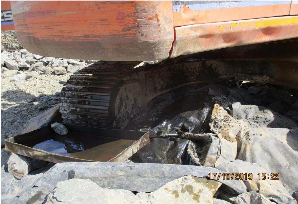
Photo: Hydraulic pipe bust from excavator (119).
